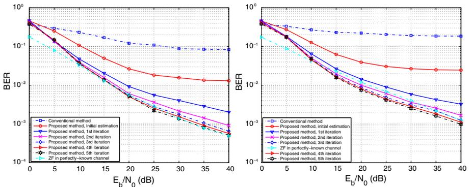
**Fig. 5** BER performances of different methods under the COST 207 BU channels. Left:  $f_d T = 0.075$ ; right:  $f_d T = 0.1$
