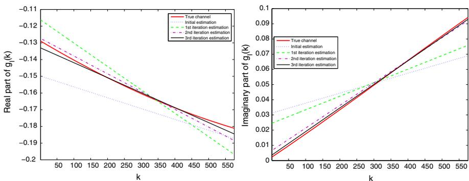
**Fig. 1** Comparisons of snapshot of path variation between true and estimated  $g_A(k)$  for  $E_b/N_0 = 40$  dB using the proposed method under COST 207 BU channels at  $f_dT = 0.1$ . A channel variation of a path across one OFDM symbol. Left: Real part; right: Imaginary part
