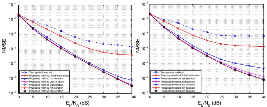
**Fig. 2** NMSE comparison of the proposed method and traditional method [8] under the COST 207 BU channels. Left:  $f_dT = 0.025$ ; right:  $f_dT = 0.05$
