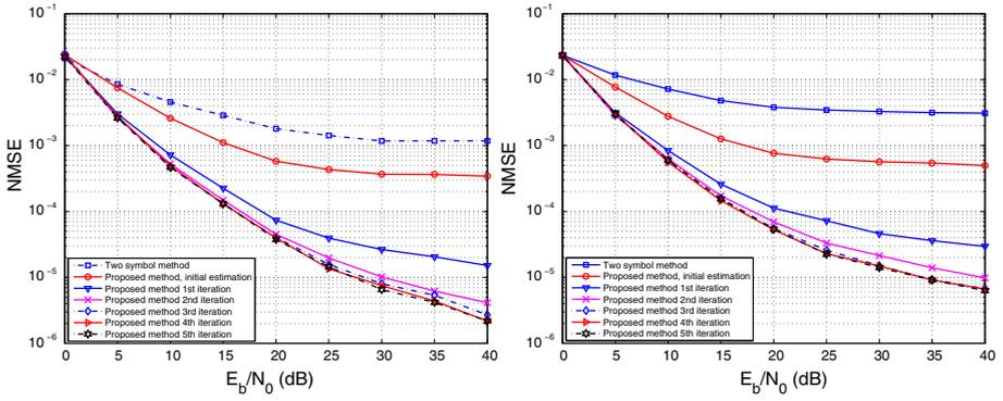
**Fig. 3** NMSE performance of the proposed and traditional methods [8] under the COST 207 BU channels. Left:  $f_d T = 0.075$ ; right:  $f_d T = 0.1$
