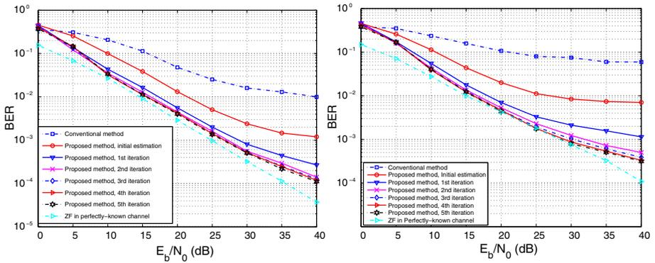
**Fig. 4** BER performances of different methods under the COST 207 BU channels. Left:  $f_d T = 0.025$ ; right:  $f_d T = 0.05$
